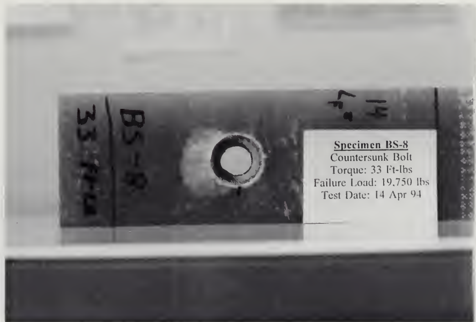
Specimen BS-8, Countersunk Bolt, 33 ft-lbs torque. View of outer GRP surface showing delamination and hole distortion. (Bolt removed from specimen.)
